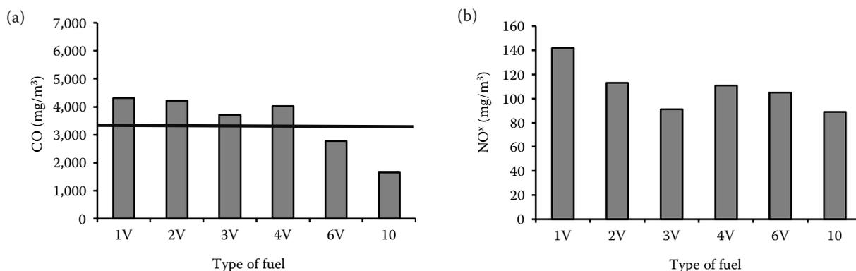
Fig. 1. Average values of gaseous CO (a) and NO<sub>x</sub> (b) emissions in flue gases of the tested forms of fuels produced from energy willow under reference O<sub>2</sub> content = 13%; emission limit of class 1 according to the standard ČSN EN 13229:2002 is designed in CO graph (black line)
