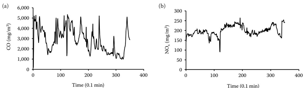
Fig. 2. Course of CO (a) and NO<sub>x</sub> (b) emissions during the combustion of briquettes from energy willows
