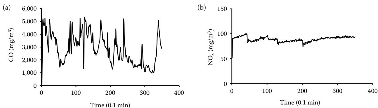
Fig. 3. Course of CO and NO<sub>x</sub> emissions during the combustion of wood briquettes Turbohard
